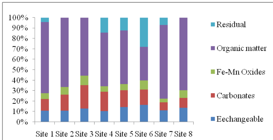
Fig. 2: Partitioning of Zn in five fraction in the road dust (<53 µm)
