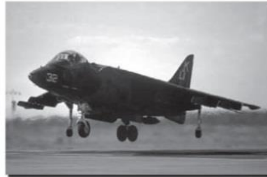
AV-8B Harrier Early 1980s 27% Composites
